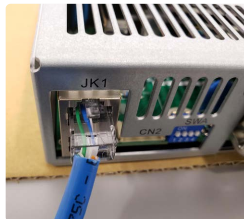
Hardware Step 2: [Ensure SDA, SCL and GND are properly connected / spliced between MCP2221A Module and DHP-1UT-B/HV Rack Shelf]
