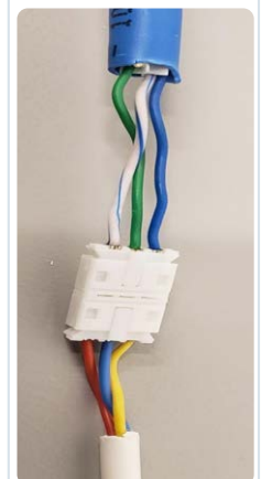
Hardware Step 2: [Ensure SDA, SCL and GND are properly connected / spliced between MCP2221A Module and DHP-1UT-B/HV Rack Shelf]
